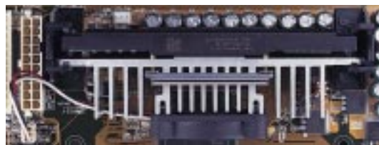
Pentium III (in an SECC2) with heatsink and fan NOTE: The SEPP fan (for Celeron processors) is similar to SECC2 fan except that the clamping design is different.
