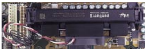
Pentium II processor packaged in an SECC with heatsink and fan (top view)
