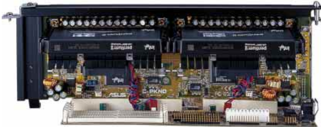
The C-PKND CPU card as assembled and installed on the baseboard.
