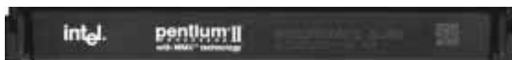
Intel Pentium II Processor in a SEC Cartridge (233-333MHz 256/512KB L2 Cache)
