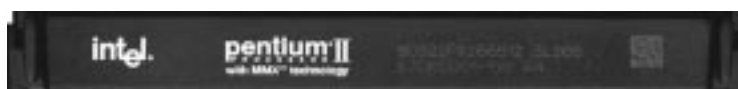
Intel Pentium II Processor in a SEC Cartridge (233-333MHz 256/512KB L2 Cache)
