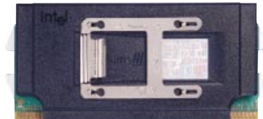
Example of an incorrectly installed retention clip
