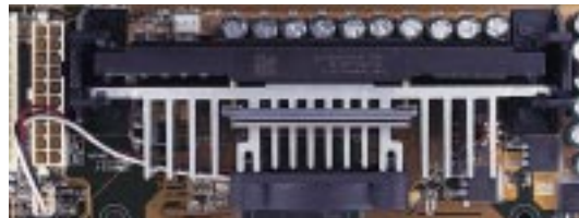
Pentium III (in an SECC2) with heatsink and fan NOTE: The SEPP fan (for Celeron processors) is similar to SECC2 fan except that the clamping design is different.
