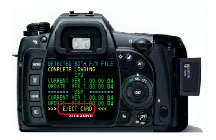
7. Remove the SD card. (Keep the memory card cover open.).
