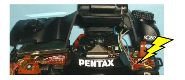
⑦ Discharging the strobe's main condenser. Lift up the A301 and discharge the electricity, charged in the main condenser, with resistance. (The white lead wire and the brown lead wire on the T750).
