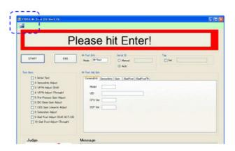
① The calibration screen appears. Click on the "Enter" key (or "START" button). (Release 15 times about for 35 secs.)
