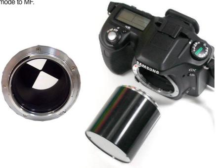
⑦ Connect the camera (Cross installation) to the EV tester.
