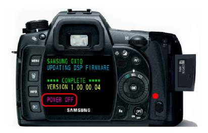
8. When the upgrade is completed, the camera's power is turned off automatically.
