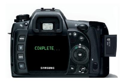
After the firmware upgrade for replacing the main board and the execution of the EEPROM PATCH are completed, make sure to carry out adjustments.
