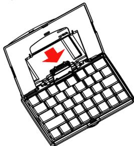
4. Pull out the left and right sections of the keyboard at the same time, until the middle section pops up.
