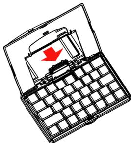
4. Pull the lid and stand together and close the cover. Press down on the cover it clicks into place.
