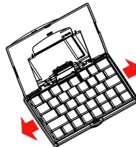
5. Push the left and right sections of the keyboard together.
