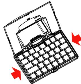
3. Flip the phone connector down until it is flush with the keyboard.
