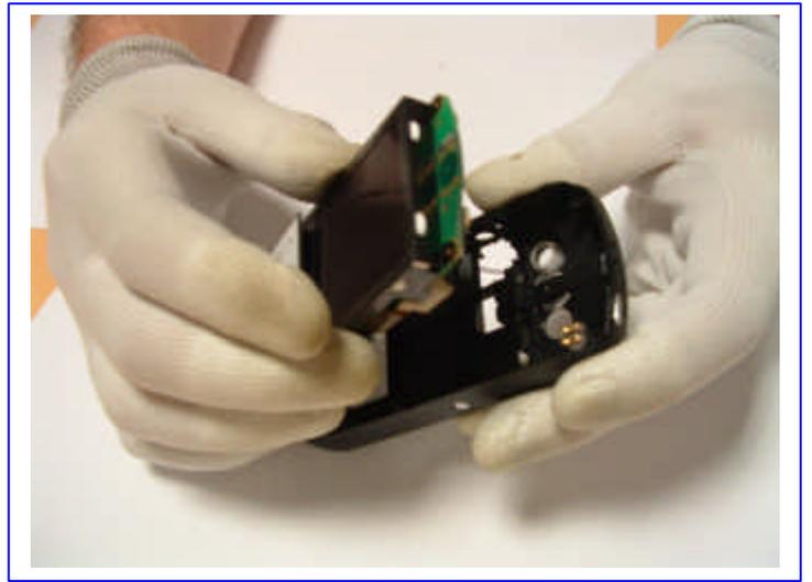
Using the opening tool insert it in the location shown opposite and gently separate the pcb from the rear cover.
