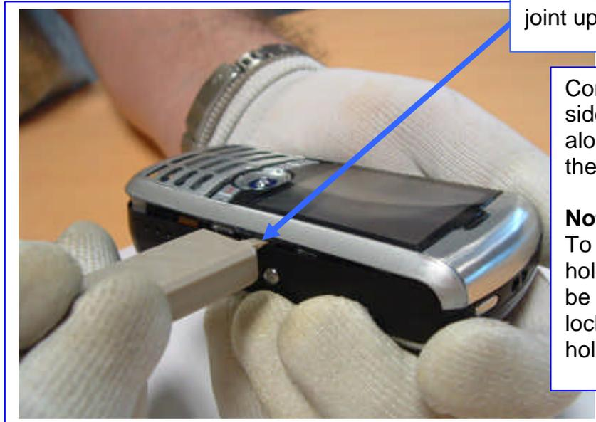
Carefully ease the covers apart along the joint up to the top of the unit.
