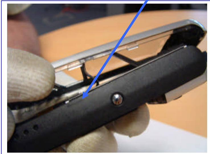
When separating the covers care must be taken when removing the LCD gasket from the LCD.
