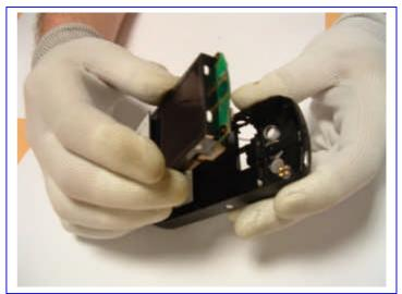
Using the opening tool insert it in the location shown opposite and gently separate the pcb from the rear cover.
