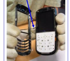
The keypad can now also be removed from the front cover.
