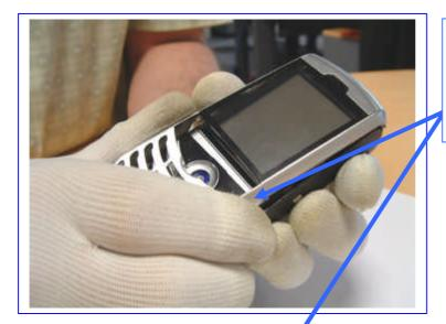
With the side locks released, gently remove the front cover from the rear cover. Start to separate the covers from the bottom first as shown.
